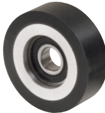
ECS H-97444 Roller, Step Trail 3" O.D. x 1" Tire Face 5/8" Bearing I.D.
